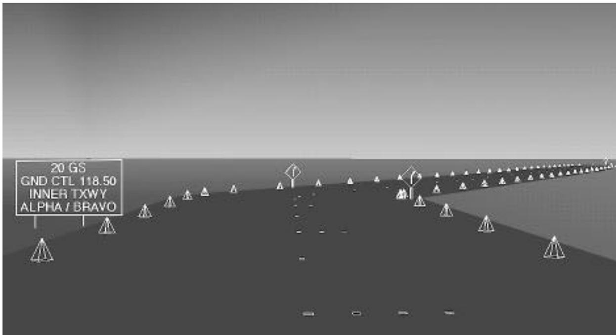
**Figure 7. Scene-linked HUD symbology for taxi and surface operations. Symbology (shown in white) includes Virtual Instruments (billboard aircraft instrumentation and location information) and virtual Scene Augmentations (edge cones, turn signs and "countdown" warnings).**
