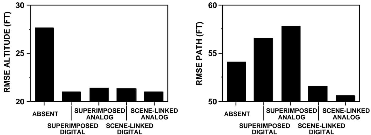
**Figure 2. Results of experimental test: Effects of HUD altitude symbology absence, superimposed digital symbology, superimposed analog clock symbology, scene-linked digital symbology and scene-linked analog clock symbology on RMSE Altitude (left) and RMSE Path right).**
