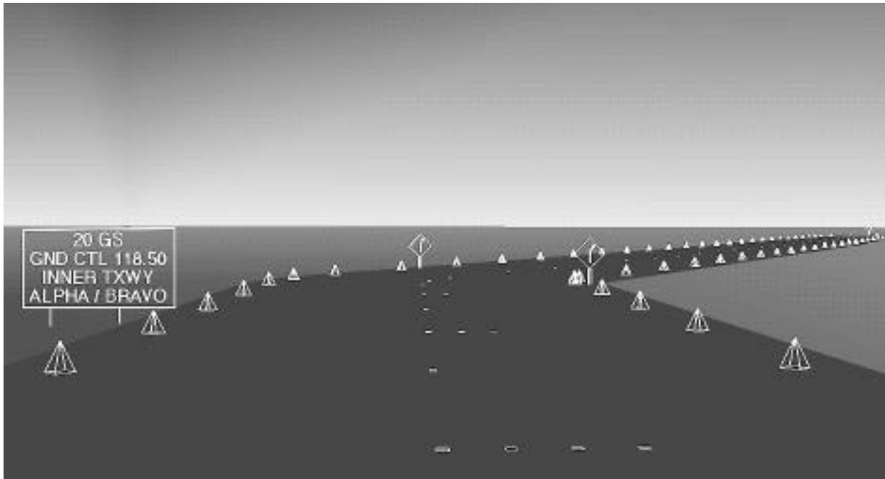
**Figure 3. Scene-linked HUD symbology for taxi and surface operations. Symbology (shown in white) includes Virtual Instruments (billboard aircraft instrumentation and location information) and virtual Scene Augmentations (edge cones, turn signs and "countdown" warnings).**
